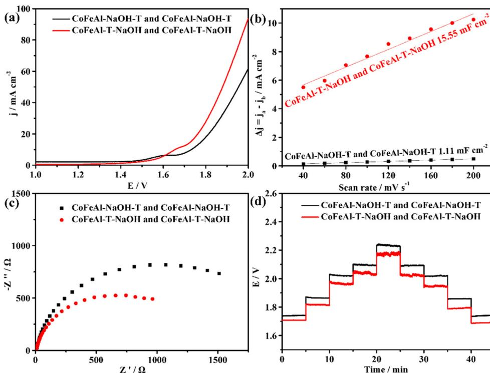
**Fig. 7** Catalytic performances of the two electrodes for overall water splitting. (a) The samples were scanned by LSV measurements at a scan rate of  $10 \text{ mV s}^{-1}$  without iR compensation. (b) The relationship between the current density difference  $\Delta j$  and the scan rate. (c) Nyquist plots measured at  $1.352 \text{ V}$  (vs. RHE). (d) Multistep chronopotentiometry response without iR compensation with current densities of  $10, 30, 75, 100$  and  $150 \text{ mA cm}^{-2}$ .
