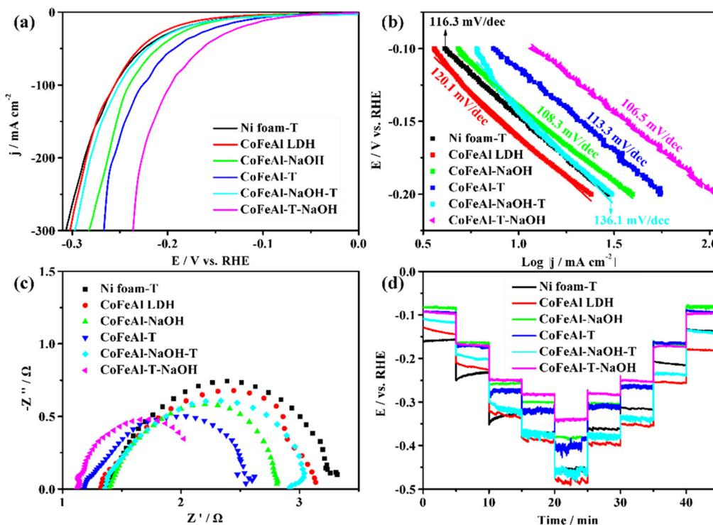
**Fig. 6** HER catalytic performances of the as-synthesized samples: (a) LSV curves at a scan rate of  $10 \text{ mV s}^{-1}$  with a 95% iR compensation. (b) The corresponding Tafel slopes. (c) Nyquist plots measured at  $-0.226 \text{ V}$  (vs. RHE). (d) Multistep chronopotentiometry response without iR compensation with current densities of  $-10, -30, -75, -100$  and  $-150 \text{ mA cm}^{-2}$ .
