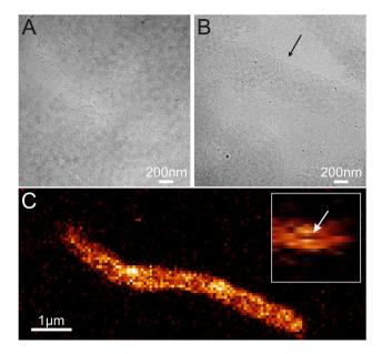
Fig. 4 Cryo-TEM and confocal microscope images of different ribbons and tubes. (A) A cryo-TEM image of 2D ribbons, (B) a cryo-TEM image of 3D tubes and (C) a side view confocal microscope image of a 3D tube. The inset in C shows the cross-section highlighted by the yellow dashed line, where a small cavity can be seen inside the tube. The size of the inset is  $2 \mu m \times 2 \mu m$ .
