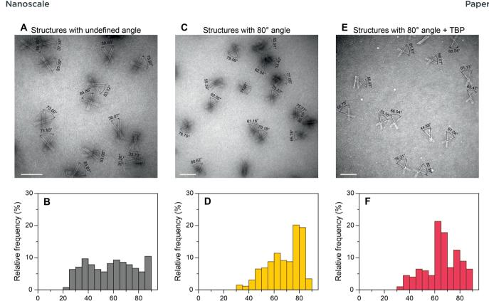
Fig. 2 TEM angle measurement and relative frequency histograms of origami structures with undefined angle (open structures) (A and B), origami structures forming 80° angle between the bundles (C and D), and origami structures forming 80° angle between the bundles incubated with 100 nM TBP (E and F). Scale bars: 100 nm.
