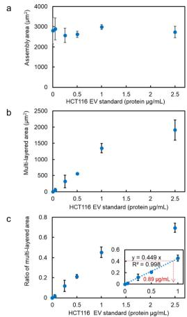
Fig. 2 Calibration curve of HCT116 standard nanoscale EVs for lightinduced acceleration in a microchannel. (a) Assembly area, (b) multilayered area, and (c) ratio of the multi-layered area at each concentration of EV standard. Inset: Low concentration range. Error bars are standard deviations (n = 3).
