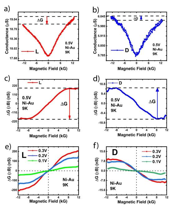
Fig. 4 (a and b) MC measurements on L and D chiral samples, respectively, in the non-linear range ( $\sim 0.5 \text{ V}$  bias). Both forward and backward field scans are recorded. Chirality dependent MC asymmetry is observed, superimposed on a symmetric background positive MC signal. (c and d) Elimination of the background MC signal and  $\Delta G$  vs. B plots. (e and f)  $\Delta G$  vs. B as a function of bias, showing that  $\Delta G$  gradually decreases with lowering bias.
