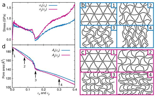
Fig. 2 Graphene foam membrane with an initial pore area of 187 Å<sup>2</sup>: (a) Stress-strain curves for loading in the x- and y-directions. Structure under increasing strain (0.005, 0.075, 0.150, and 0.300) applied in the (b) x- and (c) y-directions. (d) Pore area as a function of the strain applied in the x- and v-directions
