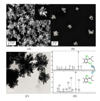
Fig. 6 (A and B) SEM and (C) TEM images of gold nanoflowers that are synthesized; mass spectral data of (D) show the process of degradation of pendimethalin (above) to N-(1-ethylpropyl)-2,6-diamino-3,4-xylidine (below). Reprinted with permission from ref. 139. Copyright © 2014, American Chemical Society. All rights reserved.
