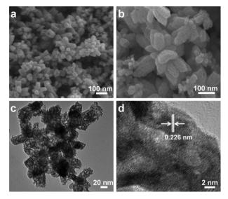
Fig. 15 SEM (a and b), TEM (c), and HR-TEM (d) images of the hnp– ${\rm Pt_{35}Cu_{65}}$  alloy. Reprinted with permission from ref. 354. Copyright © 2017 Elsevier Inc.
