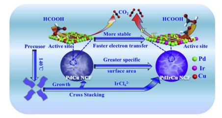
Fig. 16 Schematic illustration of the synthesis procedures and enhanced electrocatalytic performance mechanisms of the PdIrCu NCF catalyst. Reprinted with permission from ref. 360. Copyright © 2018, American Chemical Society.
