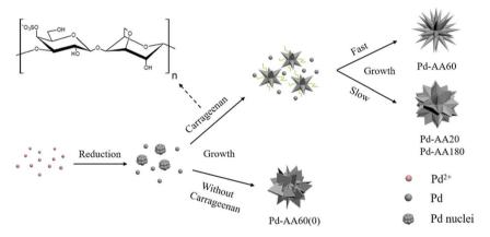
Fig. 7 Schematic illustration of the formation mechanism of Pd nanoflowers. Reprinted with permission from ref. 171. Copyright © 2017, American Chemical Society. All rights reserved.
