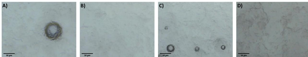
Fig. 5 Micrographs of the 1×SRA during gelation, gelation time increasing (A–D). Note higher magnification used in these images compared to blank.
