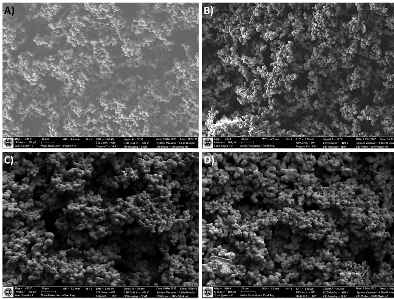
Fig. 7 Scanning electron micrographs of the cross-section surface of the un-reinforced MTMS aerogel (A) and SRA-1x (B–D).
