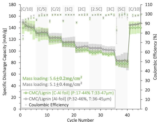
**Fig. 9** The average rate capability of three cells with aqueous produced NMC111 cathodes using CMC/lignin (green diamond) coated on plain Al-foil (empty) or carbon coated-Al-foil (C-Al) (filled).  $T$  = electrode coating thickness,  $P$  = porosity. The cathodes were cycled at different [C-rates] at  $1C = 160 \text{ mA g}^{-1}$  between 3.0 and 4.3 V (vs.  $\text{Li}^+/\text{Li}$ ) using a coin cell and Li-metal anode at  $22^\circ\text{C}$ . Calendered at  $P_{\text{medium}}$ .
