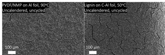
Fig. 6 SEM surface crack analysis of an uncalendered PVDF/NMP-based cathode dried at 90 °C (left) and a lignin/water-based (right) cathode dried at 50 °C with a similar mass loading ( $7.4 \text{ mg cm}^{-2} \pm 0.2$ ).
