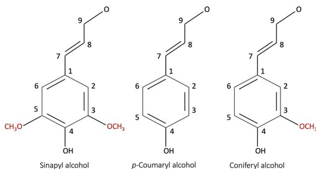
Fig. 1 The monomer species building up a lignin molecule: (a) *p*-coumaryl alcohol (4-hydroxyl phenyl, H), (b) coniferyl alcohol (guaiacyl, G), and (c) sinapyl alcohol (syringyl, S).<sup>19,26</sup>
