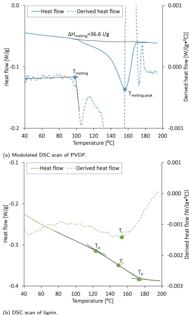
Fig. 3 Differential scanning calorimetry (DSC) measurement of (a) PVDF and (b) lignin raw materials between 30 and 300 °C.  $\Delta H_{\text{melting}}$  = heat of fusion,  $T$  = temperature,  $T_o$  = onset,  $T_i$  = inflection, and  $T_e$  = end.
