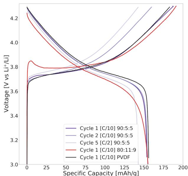
**Fig. 13** The voltage profile of the first and second cycles at  $C/10$  and the fifth cycle at  $C/2$  for NMC111 cathodes fabricated using 80:11:9 (red) or 90:5:5 (purple) lignin/water ( $7.4 \text{ mg cm}^{-2}$ ), and 85:10:5 PVDF/NMP-fabricated cathodes (black) ( $6.9 \text{ mg cm}^{-2}$ ). The cathodes were cycled in coin cells between 3.0 and 4.3 V (vs.  $\text{Li}^+/\text{Li}$ ) at different  $[C]$ -rates at 22 °C using a Li metal anode.  $1C = 160 \text{ mA g}^{-1}$ .
