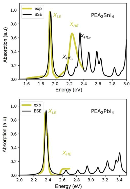
**Fig. 1** Experimental linear absorption spectrum of the polycrystalline film of (PEA)<sub>2</sub>SnI<sub>4</sub> taken at 25 K (black solid line (a)) and of (PEA)<sub>2</sub>PbI<sub>4</sub> (25 K, black solid line (b)), reproduced with permission from ref. 39). Theoretical spectra obtained via DFT+GW+BSE simulations at 0 K for (PEA)<sub>2</sub>SnI<sub>4</sub> (a) and (PEA)<sub>2</sub>PbI<sub>4</sub> (b).
