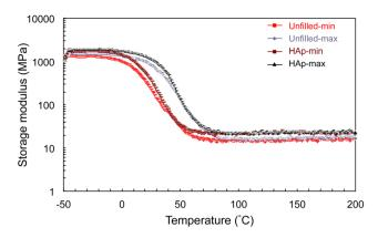
Fig. 5 The DMA curve of storage modulus and temperature demonstrated that the maximum curing condition (XVIII) was more crosslinked in both systems, demonstrated by the increase in the onset of the transition region as well as the glass transition temperature.
