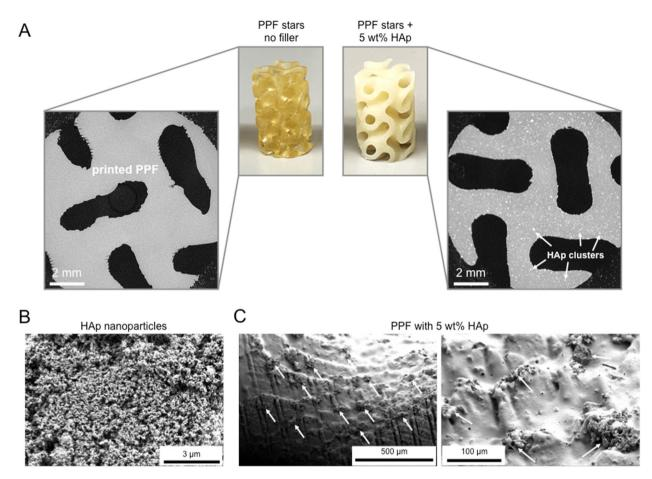
Fig. 2 Each of the printed scaffold materials was evaluated by μCT and SEM in order to observe the microstructure. (A) μCT measurements confirmed the presence of HAp clusters post-printing compared to the pure PPF. (B) HAp nanoparticles were observed with SEM to be uniform. (C) Individual HAp nanoparticles and aggregates were observed on the surface of the printed structures.
