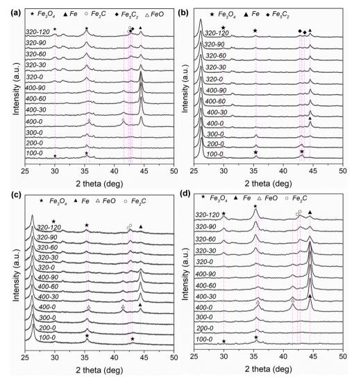
Fig. 2 In situ XRD patterns of different catalysts under given conditions: (a) K-Fe/AC-W-10, (b) K-Fe/CNF-W-10, (c) K-Fe/GA-W-10, and (d) K-Fe/ MPC-W-10. Notes: the reduction temperature was raised from room temperature to 400 °C and reduced for 90 min in a H<sub>2</sub> atmosphere, then the reaction gas was switched to reaction and phase changes were in situ detected. In terms of 320-120, 320 represents 320 °C and 120 stands for 120 min at 320 °C.
