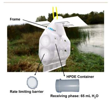
$\label{eq:Fig.1} \textbf{Fig. 1} \quad \text{The components of the equilibrium passive sampler developed} \\ \text{in this study.} \\$
