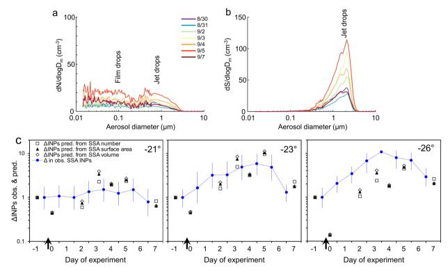
Fig. 6 Aerosol emissions over the course of the *P. marinus* addition experiment expressed on the basis of number (a) and surface area (b). (c) Observed changes in SSA INPs during the *P. marinus* experiment, expressed as the ratio of INPs on Day x with the value at the start (before the addition of detritus) compared with changes in SSA INPs predicted from  $\Delta$ INEs in the water  $\times$   $\Delta$ SSA emissions (given on the bases of aerosol number, surface area and volume).
