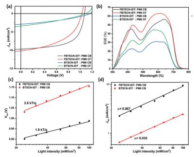
Fig. 4 J-V characteristics curves (a) and EQE spectra (b) of FBTSCN-IDT/BTSCN-IDT:PM6 blend system devices, under 1 sun. Light intensity versus (c)  $V_{\rm OC}$  and (d)  $J_{\rm SC}$  of best performance FBTSCN-IDT and BTSCN-IDT molecules-based devices
