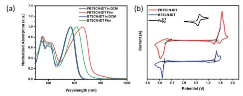
Fig. 3 (a) UV-vis absorption spectrum of FBTSCN-IDT and BTSCN-IDT in dichloromethane and film. (b) Cyclic voltammetry curves of FBTSCN-IDT and BTSCN-IDT. Measurements were taken in acetonitrile/ $[n-Bu_4N]$ PF<sub>6</sub> solutions (0.1 mol L<sup>-1</sup>). Scan rate: 0.1 V s<sup>-1</sup>.
