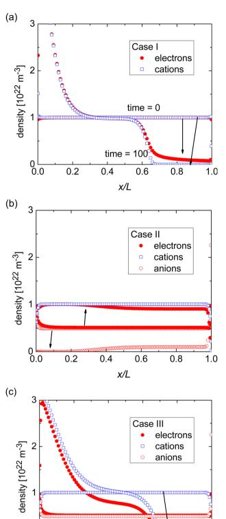
Fig. 2 Simulated profiles of the electron, cation, and anion densities for Cases I, II, and III. The arrows indicate how the density profiles change from before to after the application of the bias voltage stress.
