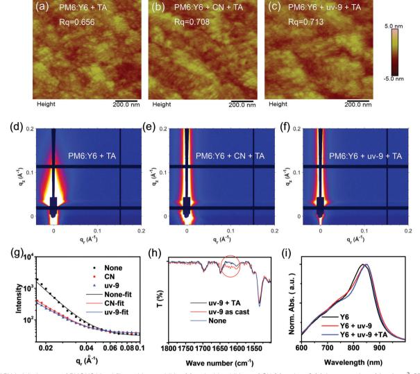
Fig. 4 AFM height images of PM6:Y6 blend films without additive (a) and with additives of CN (b) and uv-9 (c), in a scan size of  $1 \times 1 \,\mu\text{m}^2$ . 2D GISAXS images of PM6:Y6 blend films without additive (d) and with additives of CN (e) and uv-9 (f). (g) 1D in-plane intensity profiles and fitting curves of blend films with and without additive. (i) UV-vis absorption spectra of Y6 and Y6:uv-9 blend films before and after thermal annealing
