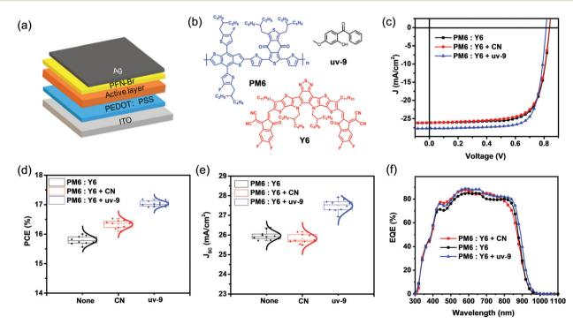
Fig. 1 (a) Schematic OSC device structure. (b) Chemical structures of PM6, Y6, and uv-9. (c) J-V characteristic curves of OSC devices with and without additives. (d) PCE statistic histogram, (e)  $J_{sc}$  statistic histogram, and (f) EQE spectra of OSCs with and without additives.
