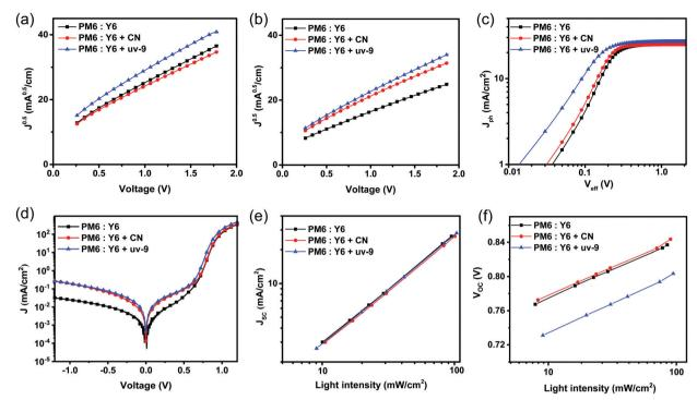
Fig. 3 (a)  $J^{0.5}-V$  curves of the electron-only devices. (b)  $J^{0.5}-V$  curves of the hole-only devices. (c) Photocurrent density ( $J_{ph}$ ) plotted against effective bias ( $V_{\rm eff}$ ) for devices without or with different additives. (d) Dark J-V curves, (e)  $J_{\rm SC}$  and (f)  $V_{\rm OC}$  versus light intensity of devices with and without additives.
