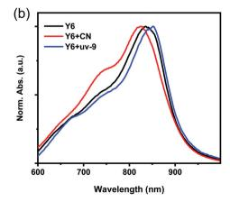
Fig. 2 UV-Vis absorption spectra of (a) PM6:Y6 blend and (b) Y6 films with and without additives
