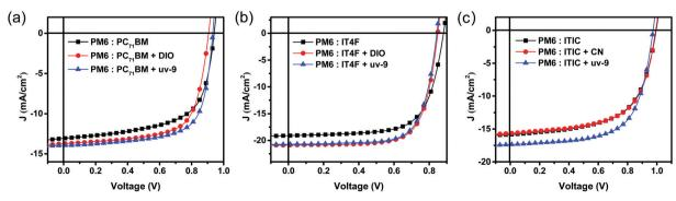
Fig. 5 J-V characteristics of (a) PM6:PC<sub>71</sub>BM, (b) PM6:IT4F, and (c) PM6:ITIC based OSC devices with and without additives
