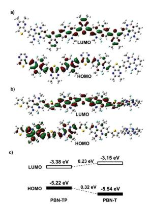
**Fig. 2** Calculated Kohn–Sham LUMOs/HOMOs based on four repeating units of (a) PBN-TP and (b) PBN-T. (c) The alignment of the LUMO/HOMO energy levels of PBN-T and PBN-TP based on DFT calculations. All the long alkyl chains have been replaced by methyl groups for simplification.
