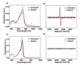
Fig. 5 UV-vis-NIR absorption spectra of (a) PBN-TP and (c) PBN-T in thin film before and after TDAE doping ( $t_{vapor} = 20 \text{ h}$ ). Electron paramagnetic resonance (EPR) spectra of (b) PBN-TP and (d) PBN-T before and after TDAE doping ( $t_{vapor} = 20 \text{ h}$ ).
