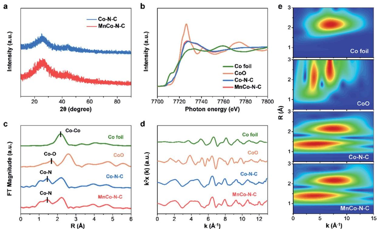
Fig. 2 Structural characterization of MnCo-N-C and controls. (a) XRD patterns. (b and c) Co K-edge XANES and EXAFS spectra, respectively. (d and e)  $k^2$ -weighted XAFS  $\chi(k)$  and wavelet transform, respectively.
