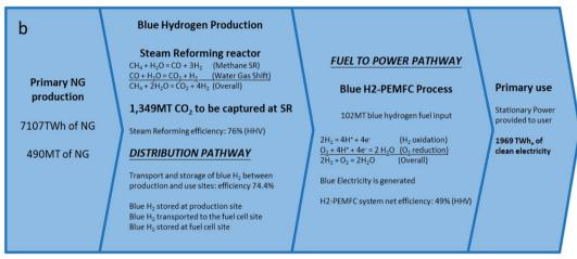
Fig. 3 Chemical and electrochemical reaction schemes for clean energy pathways involving natural gas: (a) pathway N1b: NG directly to electricity via SOFC, (b) pathway N2: NG to electricity via blue hydrogen and H2-PEMFC values are annualized predictions for 2050 following IEA's NZE scenario for 102 MT hydrogen demand for stationary FC power that equates to 1969 TW  $h_e$  electricity provided to the end user based on 49% HHV conversion efficiency.
