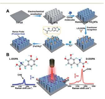
Fig. 1 (A) Fabrication of a homochiral SERS substrate and PB generation. (B) SERS-based enantiomeric recognition and qualification of DOPA enantiomers via the PB signal at 2158 cm<sup>-1</sup>.
