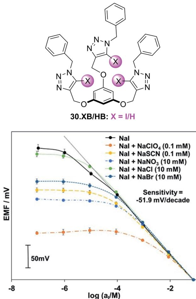
Fig. 35 Response of an ISE containing ionophore 30.XB toward iodide in the absence of presence of competing anions. Reproduced with permission from ref. 166 copyright 2021 American Chemical Society.
