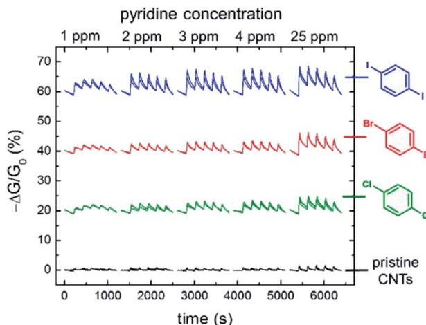
Fig. 37 Conductance response of chemiresistive gas sensors containing different dihaloaryl XB selectors in the repeating presence of increasing concentrations of pyridine in N<sub>2</sub> carrier gas. For clarity the relative conductance responses are offset by 20%. Reproduced with permission from ref. 171 copyright 2016 American Chemical Society.
