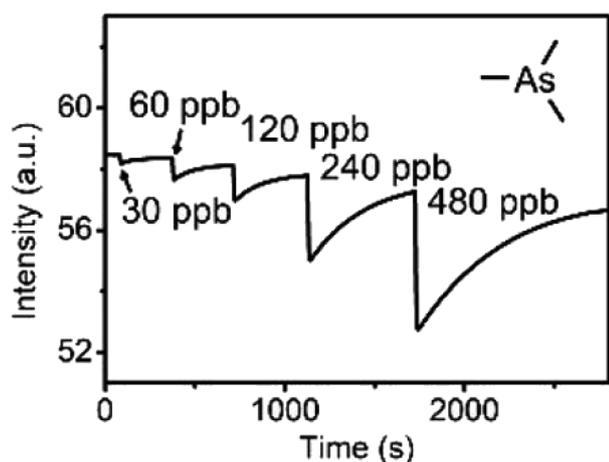
Fig. 19 Fluorescence emission intensity of bundled nanoribbons of **16.ChB** upon exposure to increasing concentration of trimethylarsine gas. Reproduced with permission from ref. 131 copyright 2021 American Chemical Society.
