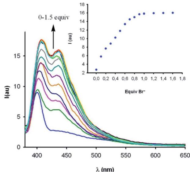
Fig. 9 Fluorescence emission response of macrocyclic iodo-imidazolium host **3c.XB** (10 μM) in CH<sub>3</sub>OH/H<sub>2</sub>O 9 : 1 in the presence of increasing concentrations of bromide. Reproduced with permission from ref. 92 copyright 2012 American Chemical Society.
