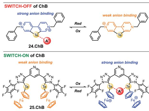
Fig. 26 ChB-mediated voltammetric anion sensing was very recently achieved for the first time as demonstrated for both reductive switch-OFF of ChB in telluroviologen **24.ChB** as well as oxidative switch-ON of ChB in pyridine bis(ferrocenyltelluroviologen) **25.ChB**.
