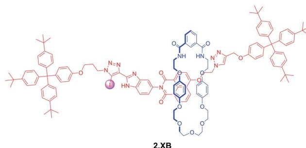
Fig. 7 XB [2]rotaxane molecular shuttle **2.XB** for colorimetric anion sensing in  $\text{CHCl}_3$ . Only in the presence of a coordinating  $\text{Cl}^-$  anion as well as acid-induced protonation of the benzimidazole does the macrocycle shuttle towards the XB anion binding site, resulting in a disruption of the hydroquinone–NDI charge-transfer interaction and a concomitant loss of colour.
