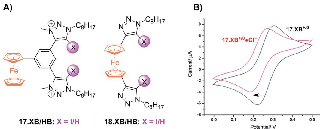
Fig. 21 (A) Chemical structures of the first XB ferrocenyl voltammetric anion sensors. (B) CVs of **17.XB** in ACN in the absence (black) and presence of 10 equiv.  $\text{Cl}^-$  (red). Adapted from ref. 141 with permission from the Royal Society of Chemistry.
