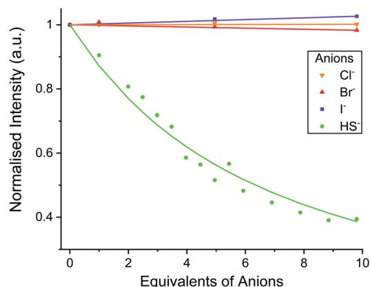
Fig. 11 Fluorescence emission intensity response of  $10\ \mu\text{M}$  hydrosulfide-selective coumarin-containing **6.XB** in the presence of 10 equiv. of various anions in 10 mM HEPES buffer (pH = 7.4). Reproduced from ref. 101 under the terms of the CC BY license.
