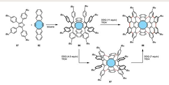
Scheme 24 Synthesis of an [8] circulene derivative 88 containing 80 sp<sup>2</sup> carbons by reaction of naphthannulated cyclooctadiyne 82 with cyclopentadienone 57 via two-fold Diels-Alder cycloaddition and Scholl reaction.
