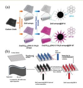
Fig. 5 (a) Scheme showing the synthetic process of ZnO@ZIF-8 and Co (CO<sub>3</sub>)<sub>0.5</sub>(OH)·0.11H<sub>2</sub>O@ZIF-67 on CC. Reprinted with permission from ref. 63, Copyright 2018, American Chemical Society. (b) Schematic illustration showing the fabrication of ZnO@ZIF-8 derived nanotubes. Reprinted with permission from ref. 64, Copyright 2018, Elsevier.
