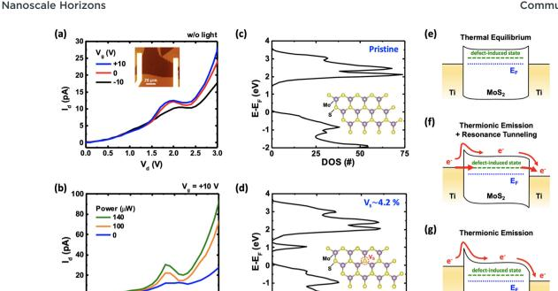
Fig. 4 (a)  $I_d - V_d$  curves at different gate voltages without light illumination. The inset presents the OM image of the measured device. (b)  $I_d - V_d$  curves illuminated with different light power values at a fixed gate voltage  $V_0 = +10 \text{ V}$ . (c and d) Density of states (DOS) of pristine monolayer MoS<sub>2</sub> and that with  $V_{\rm S} \approx 4.2\%$ , respectively. (e-g) Schematics of band diagrams for different stages of the NDR mechanism.
