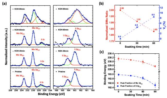
Fig. 2 (a) X-ray photoemission spectroscopy (XPS) of Mo 3d (left panel) and S 2p (right panel) at various KOH soaking times. (b) Normalized S/Mo ratio and S-vacancy ( $V_S$ ) as a function of soaking time showing an increasing percentage of  $V_S$  with increasing soaking time. (c) Peak positions of Mo  $3d_{5/2}$  and S 2p<sub>3/2</sub> shift to lower binding energy values with increasing soaking time.
