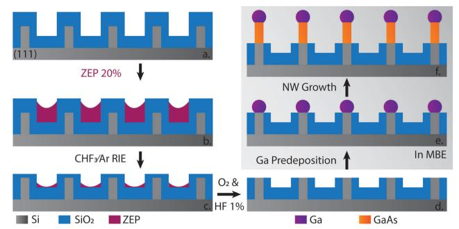
Fig. 1 Schematic detailing the fabrication steps of SiO<sub>2</sub>/Si(111) pillars for self-catalyzed VLS GaAs NW growth. (a and b) The resist spin-coating process, (b and c) The RIE step and (c and d) the last wet etching before MBE loading. (e) Shows the very critical Ga predeposition step followed by (f) showing NW growth.
