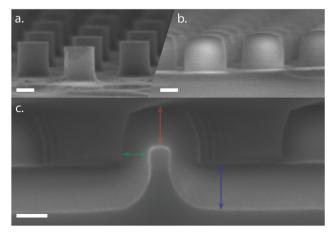
Fig. 6 SEM images showing (a) PSL-patterned Si pillars after RIE, (b) after 70 nm nominal dry oxidation and (c) a cross-section of a SiO<sub>2</sub>/Si pillar after 160 nm dry oxidation. Scale bars are 100 nm.
