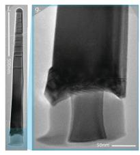
Fig. 7 Self-catalyzed VLS growth of GaAs NWs on SiO<sub>2</sub>/Si (111) PSL pillars. (a) Large-scale array showing a 40% vertical yield. (b) Local vertical yield of 67% from a spin-coating comet. (c-e) TEM bright-field images of ZB and WZ nanowires coming from the same  $SiO_2/Si$  large-scale array. The WZ FFT is visible. (f and g) WZ GaAs NW and the  $SiO_2/Si$  pillar where it grew from. The pillar's Si core and  $SiO_2$  shell are visible.
