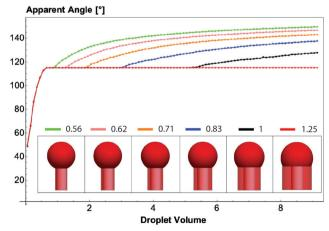
Fig. 5 Results of simulations done on Surface Evolver™. The graph shows the droplet apparent angle, i.e. contact angle, for  $d_{SiO_2}/d_{Si}$  ratios of 0.56, 0.62, 0.71, 0.83, 1 and 1.25.
