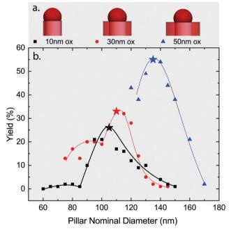
Fig. 4 (a) Schematics showing the change in  $SiO_2/Si$  pillar nominal diameter for a fixed Si core diameter and Ga dropelt volume. (b) Vertical yield as a function of the SiO<sub>2</sub>/Si pillar nominal diameter for nominal oxidations of 10 nm, 30 nm and 50 nm.
