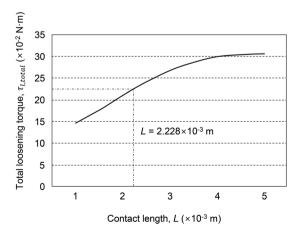
Fig. 11 The effect of contact length, L, on the total loosening torque,  $\tau_{l,total}$ . This graph shows total loosening torque values, based on the data in Table 1.
