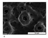
Fig. 4 (A) Scanning electron microscopy (SEM) image of a hydrophilic SLA surface (SLActive, Institute Straumann AG, Basel, Switzerland). There are no distinct differences in specific SEM features between hydrophilic and standard SLA surfaces. (B) SEM images of an anodically oxidized Ti surface (TiUnite, Nobel Biocare, Zürich, Switzerland) displaying protruded open pore micro-structures.
