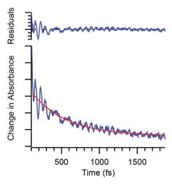
Fig. 3 Time-resolved absorption data for  $Cr(acac)_3$  following ca. 40 fs excitation into the  $^4A_2 \rightarrow ^4T_2$  ligand-field absorption at  $\sim$ 550 nm. The oscillatory features are due to quantum oscillations associated with electronic state evolution in this compound.
