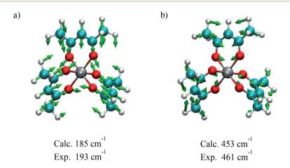
Fig. 12 Nuclear displacements associated with the coherent oscillations shown in Fig. 11 at (a) 193 cm<sup>-1</sup> and (b) 461 cm<sup>-1</sup>. The modes were visualized based on DFT calculations that yielded the energies indicated, whereas the experimental numbers reflect averages over multiple data sets.
