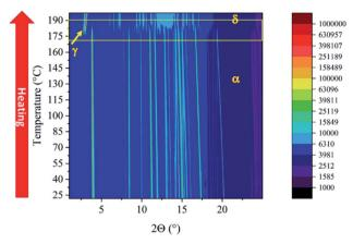
Fig. 3 VT-XRPD of NDI-C6 at PSI synchrotron, 2D isolines of first heating until 195 °C with a transition of Form  $\alpha \to$  Form  $\delta$  at 180 °C, and the presence of the Form  $\gamma$  peak is highlighted with an arrow.
