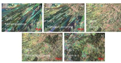
Fig. 4 Hot stage microscopy during the cooling after the melting of a single crystal NDI-C6, (a) recrystallization at 203 °C into Form  $\delta$ , (b) Form  $\delta \to \text{Form } \gamma$  transition starting at 160 °C, (c) transition into Form  $\gamma$  completed, (d) transition Form  $\gamma \to \text{Form } \alpha$  occurring at 145 °C, (e) transition into Form  $\alpha$  completed.
