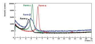
Fig. 7 Thin films of the different phases, identified by the characteristic peak of each phase, Form  $\alpha$  in red, Form  $\beta$  in blue, Form  $\gamma$  in black and Form  $\epsilon$  in green.
