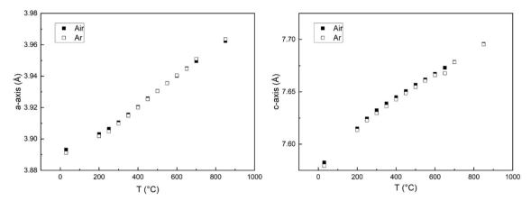
Fig. 14 Cell parameters for a-axis (left) and c-axis (right) vs. temperature for x = 0 in air (closed squares) and Ar (open squares) atmospheres.
