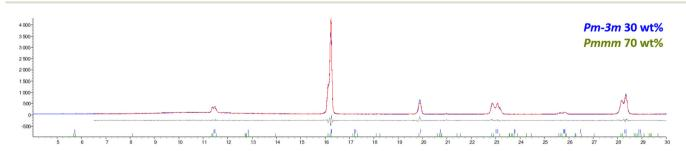
Fig. 4 SR-PXD with rietveld refinement of reduced, partly A-site ordered BLC
