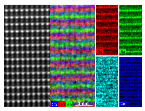
Fig. 11 STEM dark-field image (left) and EDS elemental mapping (middle and right) of BGLC82 in dry state.
