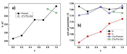
Fig. 5 Unit cell volume (a) and cell parameters (b) for BGLC (x = 0, y = 0-1).
