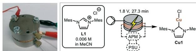
**Fig. 1** Miniaturised electrochemical flow reactor comprising circular stacked electrodes (48 mm diameter) separated by PTFE spacers (1 mm thick) with flow channels of 0.464 mL. Model electrochemical reaction; synthesis of Cu1 from L1 and copper electrodes.
