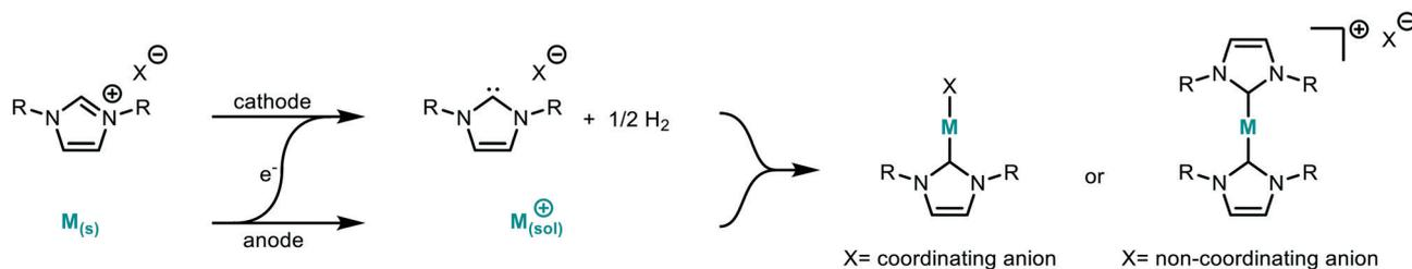
**Fig. 2** Electrochemical synthesis of metal-NHC complexes. An imidazolium salt is reduced at the cathode to form the NHC with concomitant oxidation of the sacrificial anode to produce metal ions to which the NHC coordinates.
