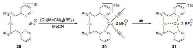
Scheme 9 Synthesis of dinuclear heterometallic compounds **29**–**31** with PPy ligand ( $L^{11}$ ).<sup>55</sup>
