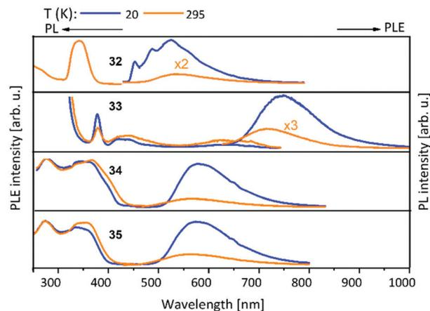
Fig. 10 Solid state excitation and emission spectra of PN<sub>4</sub> (**L**<sup>12</sup>) metal complexes **32**–**35**. PL was excited at  $\lambda_{\text{exc}} = 350$  nm and PLE spectra recorded at  $\lambda_{\text{em}} = 560$  nm for **32**, **33**, **35** and  $\lambda_{\text{em}} = 580$  nm for **34**.<sup>48</sup>
