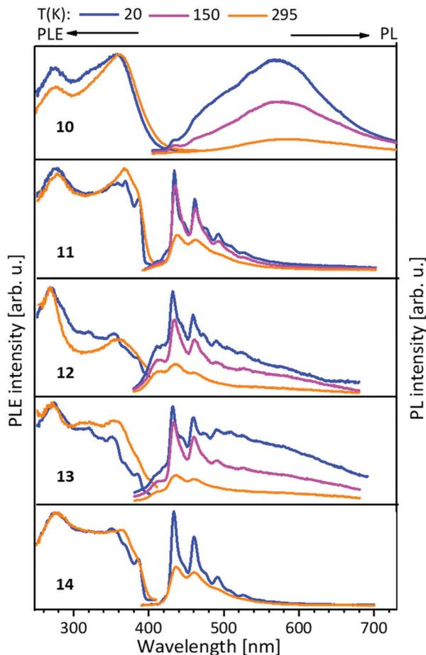
Fig. 7 Solid state excitation and emission spectra of NHC<sup>impy</sup> ( $L^3$ ) metal complexes **10–14**. PL was excited at  $\lambda_{exc} = 350$  nm and PLE spectra recorded at  $\lambda_{em} = 580$  nm for **10** and  $\lambda_{em} = 430$  nm for **11–14**,  $\lambda_{em} = 430/460$  nm (**13**).<sup>43</sup>
