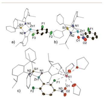
Fig. 3 Crystal structures of: (a) anion of 3a; (b) anion of 3d; and (c) 3e. Thermal ellipsoids are rendered at 50% probability. Hydrogen atoms and minor disorder components are omitted and Ph and Ar\* fragments and THF molecules are drawn as wire frames for clarity
