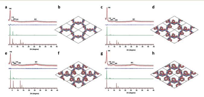
Fig. 1 Powder XRD patterns of experimental (black), Pawley-refined (red), their difference (blue), simulated eclipsed (green) and staggered (brown) stacking for (a) COF20Me, (c) COF15C5, (e) COF18C6 and (g) COF21C7. Simulated crystal structures of (b) COF20Me, (d) COF15C5, (f) COF18C6 and (h) COF21C7.
