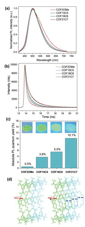
Fig. 2 (a) Solid state photoluminescence spectra, (b) fluorescence decay curves, (c) absolute fluorescence quantum yield with inset fluorescence images of COF2OMe, COF15C5, COF18C6 and COF21C7 powders. (d) Schematic presentation of backbone rotation restriction by stacking of semi-rigid crown ether chains (red arrow indicates possible rotation mode, blue arrows represent repulsion force).
