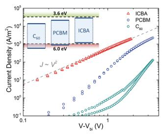
Fig. 11 Current density vs. voltage characteristics of ICBA (213 nm), [60]PCBM (222 nm), and C<sub>60</sub> (227 nm) hole-only devices, corrected for the built-in voltage ( $V_{\rm bi}$ ). The grey dashed line indicates a quadratic voltage dependence. The inset shows a schematic energy diagram, indicating the IE and EA of the fullerene derivatives with respect to the trap-free window (dashed lines) (reprinted by permission from Macmillan Publishers Ltd: Nat. Mater., ref. 45, copyright 2019).
