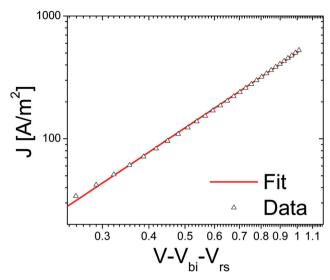
**Fig. 6** Current density vs. voltage, corrected for built in voltage and series resistance of a bisPCBM electron only device. Data (symbols) is fitted (solid line) using a space charge limited current with a mobility of  $7 \times 10^{-8}$  m $^2$  V $^{-1}$  s $^{-1}$  (reprinted with permission from ref. 30. Copyright 2008 Wiley-VCH Verlag GmbH & Co. KGaA, Weinheim).
