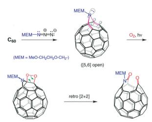
Fig. 1 Azafulleroid conversion to "holey bucky".6
