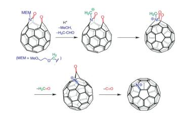
Fig. 2 Formation of heterofullerene C<sub>59</sub>N.<sup>7</sup>
