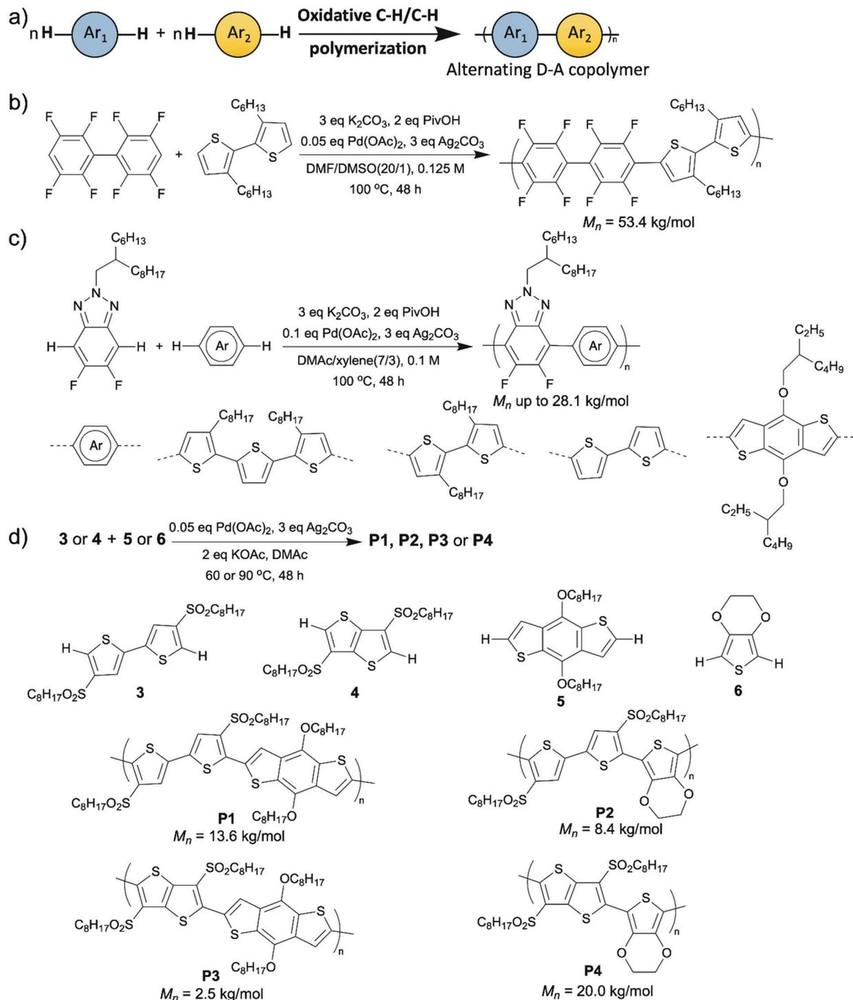
**Scheme 8** (a) A general synthetic scheme of D–A semiconducting copolymers *via* CDC. (b) Palladium/silver catalyzed CDC polymerization. (c) Synthesis of fluorinated benzotriazole containing D–A conjugated copolymers *via* CDC. (d) The CDC polymerizations of various D–A conjugated copolymers.
