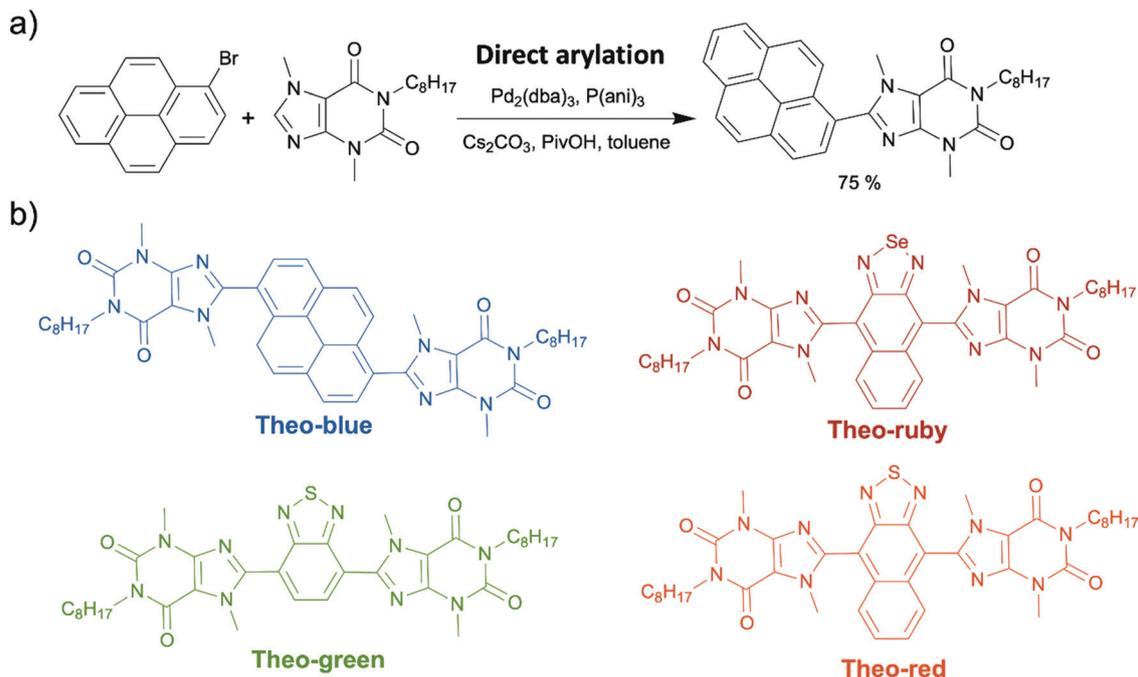
**Scheme 16** (a) Direct arylation to attach alkylated theobromine onto pyrene. (b) The structures of the four synthesized theobromine-based organic dyes (Theo-blue, Theo-green, Theo-ruby, and Theo-red).
