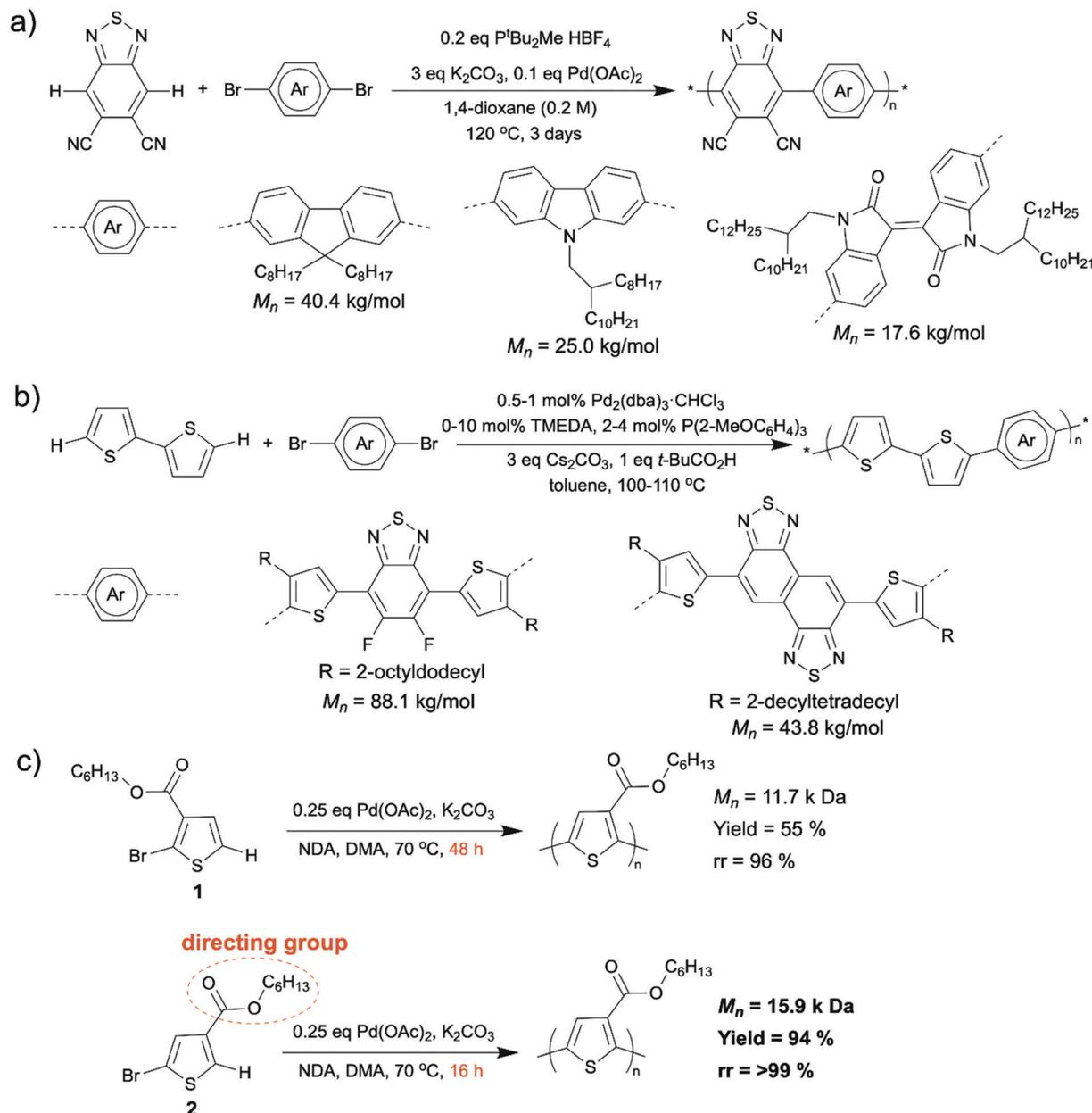
**Scheme 5** (a) Synthesis of DCBT containing conjugated D–A copolymers via DARP. (b) Synthesis of unsubstituted bithiophene containing D–A copolymers via DARP using a mixed ligand catalyst to suppress branching side reactions. (c) Synthesis of highly regioregular P3HET via DARP with the ester functionality as the directing group to promote regioregularity.
