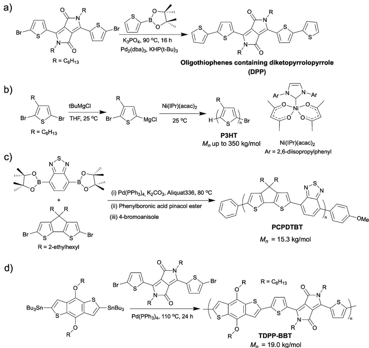
**Scheme 1** (a) Synthesis of diketopyrrolopyrrole (DPP) containing oligothiophenes via Suzuki coupling.<sup>12</sup> (b) Synthesis of P3HT via Kumada catalyst transfer polycondensation (KCTP).<sup>13</sup> (c) Synthesis of poly[4,4-bis(2-ethylhexyl)-4Hcyclopenta[2,1-b:3,4-b']dithiophene-2,6-diyl-alt-2,1,3-benzothiadiazole-4,7-diyl] (PCPDTBT) via Suzuki coupling.<sup>14</sup> (d) Synthesis of DPP containing copolymers (TDPP-BBT) via Stille coupling.<sup>15</sup>
