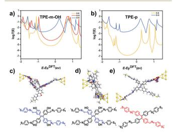
Fig. 4 (a and b) Calculated transmission spectra for TPE-m-OH (a) and **TPE-p** (b) with different anchoring sites. (c-e) The transmission path for  $S_1-S_4$  (c), the  $N_1-N_4$  anchoring site of **TPE-m-OH** (d), and the  $S_1-S_4$ anchoring site of TPE-p (e).
