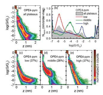
**Fig. 3** (a) 2D histogram for **OPE4-pym** build from all traces displaying plateaus, (b) 1D histogram for all traces displaying plateaus of **OPE4-pym** (grey background) and those corresponding to low (red), middle (green) and high (blue) conductance after clustering analysis, (c), (d), and (e) 2D histograms of the three different groups of plateaus obtained after the clustering-based analysis method.
