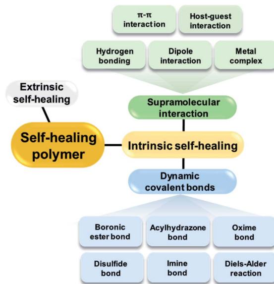
Fig. 1 Strategies used to prepare self-healing polymers.
