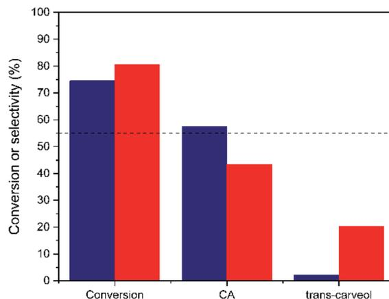
Fig. 9 Conversion and different product selectivities obtained for the  $\alpha$ -pinene oxide isomerization when using Hf-MOF-808\_H<sub>2</sub>O (red bar) and Hf-MOF-808\_DMF (blue bar) as catalysts.
