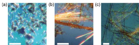
Fig. 2 Polarized optical microscopy (POM) images of (a) **TPHAT-P**, (b) **TolHAT-1**, and (c) **ThiaHAT-1** under daylight. Scale bar: 100 μm.
