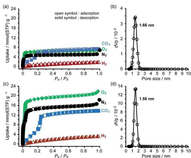
Fig. 7 (a and c) Gas sorption isotherms and (b and d) pore distribution of (a and b) **TolHAT-1aIV** and (c and d) **ThiaHAT-1a**. The isotherms were recorded at  $-196^\circ\text{C}$  for  $\text{N}_2$ ,  $\text{O}_2$ , and  $\text{H}_2$  and at  $-78^\circ\text{C}$  for  $\text{CO}_2$ . Solid and open symbols denote absorption and desorption processes, respectively.
