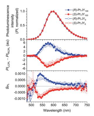
Fig. 5 Circularly polarized luminescence of JY films doped with 30 wt% Pt dopants. Top, Photoluminescence spectra; middle, circularly polarized luminescence spectra; bottom, the variations in  $g_{\rm Pl}$  with wavelength.
