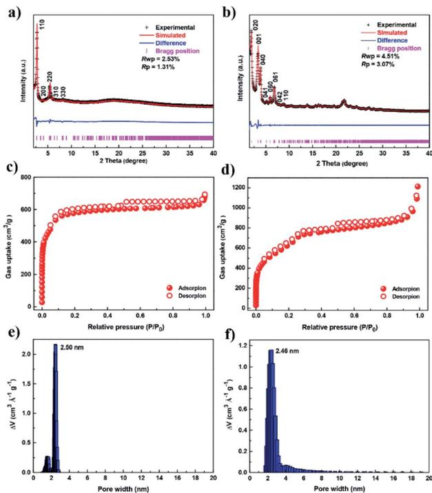
**Fig. 2** PXRD profiles and porosity. (a and b) PXRD patterns of JUC-560 (a) and JUC-561 (b). (c and d)  $N_2$  adsorption–desorption isotherms of JUC-560 (c) and JUC-561 (d) at 77 K. (e and f) Pore-size distribution of JUC-560 (e) and JUC-561 (f) calculated by fitting on the NLDFT model to the adsorption data.
