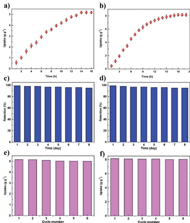
**Fig. 3** Study of iodine capture. (a and b) Uptake of iodine of JUC-560 (a) and JUC-561 (b) as a function of exposure time at 75 °C and ambient pressure. (c and d) Iodine retention of the iodine-captured JUC-560 (c) and JUC-561 (d) upon exposure to air at 25 °C and ambient pressure. (e and f) Recyclability of JUC-560 (e) and JUC-561 (f) in iodine adsorption.
