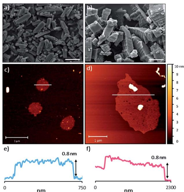
Fig. 3 (a) and (b) SEM images of bulk **1** and **2·TP** respectively. Scale bars represent 10 μm. (c) and (d) selected AFM topographical images of the nanosheets formed from exfoliation of **1** and **2·TP** respectively. (e) and (f) height profiles of the nanosheets shown in (c) and (d) (represented by white bars).
