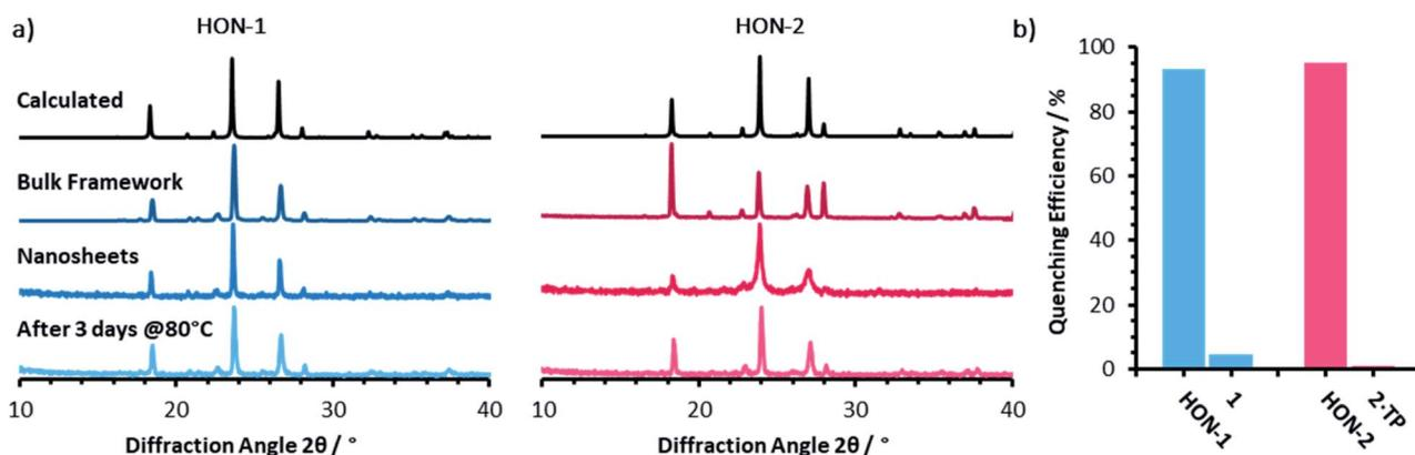
Fig. 4 (a) Powder X-ray diffractometry patterns for both the one (blue) and two (pink) component systems, of: the calculated and as synthesised frameworks, nanosheets, and water treated nanosheets. (b) The quenching efficiencies of hydrogen-bonded framework nanosheets and bulk frameworks towards Rhodamine B fluorescence ( $\lambda_{\text{ex}} = 556$ ,  $\lambda_{\text{em}} = 577$  nm). Emission titration spectra can be seen in Fig. S21–S24.<sup>†</sup>
