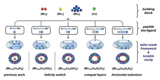
Scheme 1 Schematic representation of peptide sequence mediated self-assembly processes for bio-hybrid MB nanowheels with tailor-made architectures.
