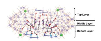
Fig. 1 Molecular structure of  $\{Mo_{124}Ce_4(GH)_4\}$ . Color code: green, Ce; blue, Mo; red, O; pink, N; grey, C; navy line,  $\{Mo_2\}$  units. Coordination bonds (sky blue line) and hydrogen bond networks (orange dash) between four GH and MB framework are highlighted in the cavity, while the oxygen atoms on MB are omitted for clarity.
