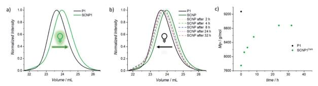
Fig. 1 (a) Normalized UV-SEC-trace at 250 nm of the crosslinker mediated folding of P1 (black line) with BisTAD using green light ( $\lambda_{max} = 525$ nm). The resulting collapsed polymer chain is displayed in dark green (SCNP1). (b) Normalized UV-SEC-traces at 250 nm of the stepwise unfolding process of SCNP1 over time in the dark. (c) Evolution of M<sub>P</sub> during the stepwise unfolding process over time of SCNP1.
