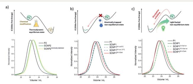
Fig. 2 Schematic display of hypothetic energy landscapes (top) and normalized UV-SEC traces (bottom) of the (a) kinetically trapped nonequilibrium macromolecular architecture, (b) chemically stabilized folded macromolecular architecture, and (c) light-fueled stabilization of the non-equilibrium macromolecular architecture
