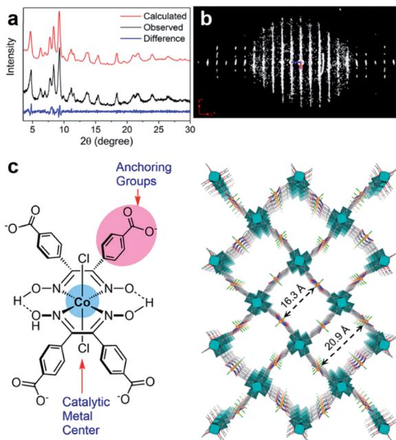
Fig. 11 (a) Pawley fitting profiles of the PXRD pattern of UU-100 ( $\lambda = 1.5418$  Å). (b) 3D reciprocal lattice of UU-100 reconstructed from 3DED data. (c) Structure of the cobaloxime linker, and the structural model of UU-100 showing open reticular pore structures.<sup>92</sup> Reproduced from ref. 92 with permission from the American Chemical Society, copyright 2019.
