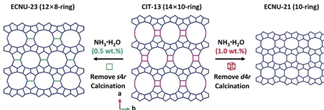
Fig. 4 Structural transformation from germanosilicate CIT-13 into high silica zeolites ECNU-21 and ECNU-23.<sup>57</sup> The structures of all three zeolites were discovered by cRED. Reproduced from ref. 57 with permission from the John Wiley & Sons, Inc., copyright 2020.
