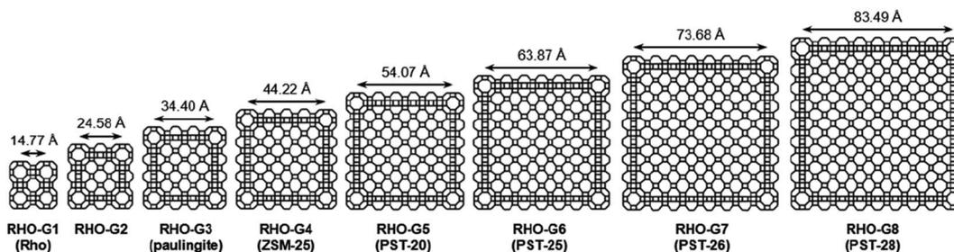
Fig. 6 Framework representations of cross sections (ca. 12 Å thick) of RHO-G1 to RHO-G8 in the RHO family of embedded isorectical zeolites.<sup>66</sup> Reproduced from ref. 66 with permission from the John Wiley & Sons, Inc., copyright 2016.
