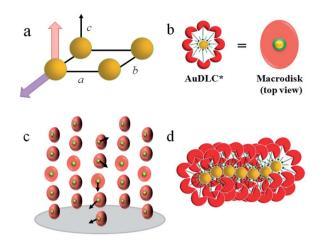
Fig. 2 Schematic representation of (a) p2 lattice with parameters a=4.17 nm, b=2.52 nm and the angle  $\gamma \sim 48.4^\circ$ ; spatial direction c not defined by the lattice. Red arrow:  $N_{\rm D}^*$  helix axis; purple arrow: plasmonic interactions. (b) AuDLC\* macrodisk. Yellow: gold core; red: PA unit; green: chiral sheath. (c)  $N_{\rm D}^*$  phase formed by functionalized NPs. (d) Chiral assembly behaviour of gold NPs along the axis of smallest lattice parameter b.
