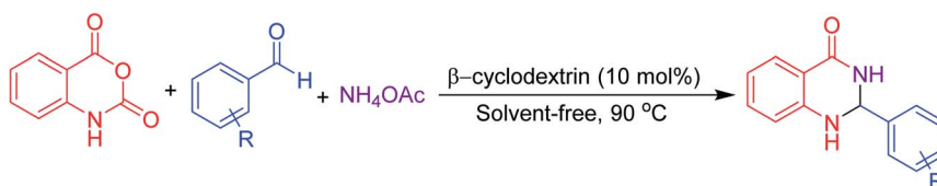
Scheme 2 One-pot three-component synthesis of 2,3-dihydroquinazolin-4(1 H )-one.
